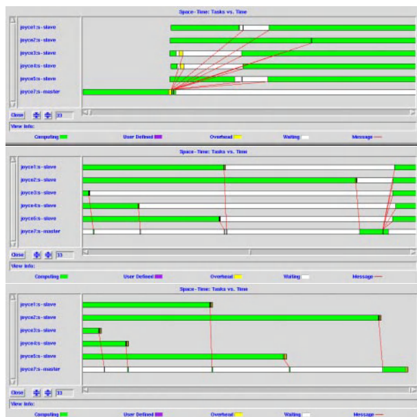
Fig. 3. Illustration of a typical parallel behaviour of the algorithm running on cluster of Pentium workstations under PVM.
